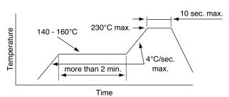
The following soldering patterns are recommended for reflow soldering
